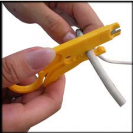
STEP 1 Place UTP/STP cable on tool
