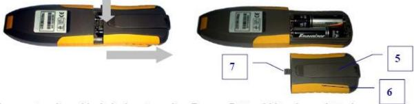
To press to release Linchpin then to push Battery Lid backward.
