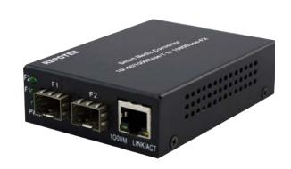
and 100/1000Base-X network. With the two 100Base-FX or 1000Base-SX / LX SFP ports, the RP-MC312FP provides high reliability and flexibility to extend the media transmission distance up to 550m, 20km, or longer depending on the SFP fiber modules. It allows the two types of segment to connect easily, efficiently and inexpensively.
