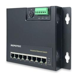
With its unique flat and wall-mounted cabinet design fits easily in any space-limited location, such as a shallow cabinet or a small enclosure.
