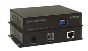
over single pair copper line for point-to-point Ethernet connectivity. With 100/60Mbps data rate, RP-VC102EP supports transmission distance up to 300 meters, and 30/10 Mbps for 1km long range connection. Users may also select a fixed data rate or a fixed SNR margin for different copper line ranging. With Power Sourcing Equipment, RP-VC102EP provides power supply over Ethernet cable to the 802.3af compliant power device.
